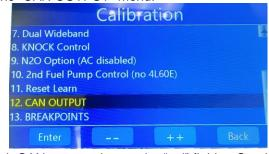
• For each CAN output, change the "val" field to On, then press the "Send to ECU" button to turn the output on.
