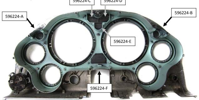
4. Using the 10 factory screws from Step One, secure the Dakota Digital gauge assembly to the bezel.
