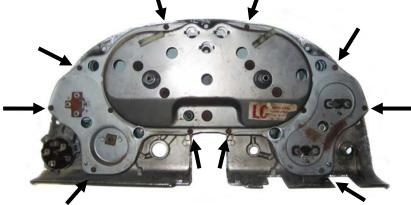
2. Remove the stock gauges. To remove the lens separator plate, remove these eight nuts (white arrows). The only item to be reused is the original front bezel; the other pieces can be discarded. Now is a good time to clean the bezel and remove any dirt or old lens gasket material.
