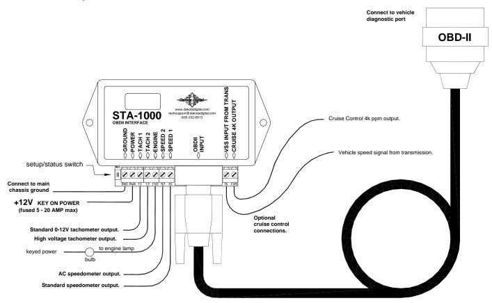
This unit has an input to read engine information from vehicles using the GM 1996-up OBD-II protocol, Ford 1996-up OBD-II protocol, some Chrysler 2000-up OBD-II protocol, or CAN OBD-II protocol. CAN OBD-II is used on all vehicles 2008 and newer and some vehicles from 2004 – 2008. It provides speedometer, tachometer, and engine indicator outputs. Do not mount this in the module in the engine compartment; it should be mounted in interior of the vehicle.
