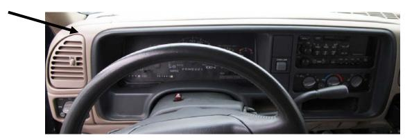
1b. Remove the four screws securing the gauge cluster to the dash. Unplug and remove the gauge cluster.
