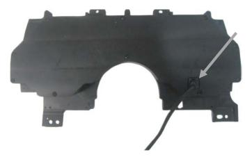
6. Mount the VHX gauge to the dash using the four (4) factory screws.
