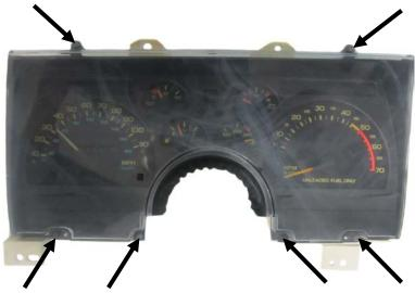
3. The inner gauge panel and column dust seal will be reused so remove the six (6) screws that secure the clear lens and also the additional three (3) screws on top that mounts the inner gauge panel. Save all hardware for reassembly.
