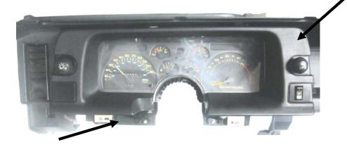
Remove the stock gauge cluster from the dash by removing the four (4) screws, retain the hardware for reassembly.
