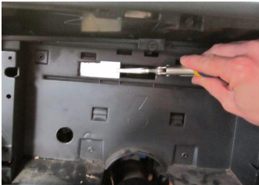
Use locking pliers to hold the cut guard into place to protect the harness from damage while cutting the inner structure
