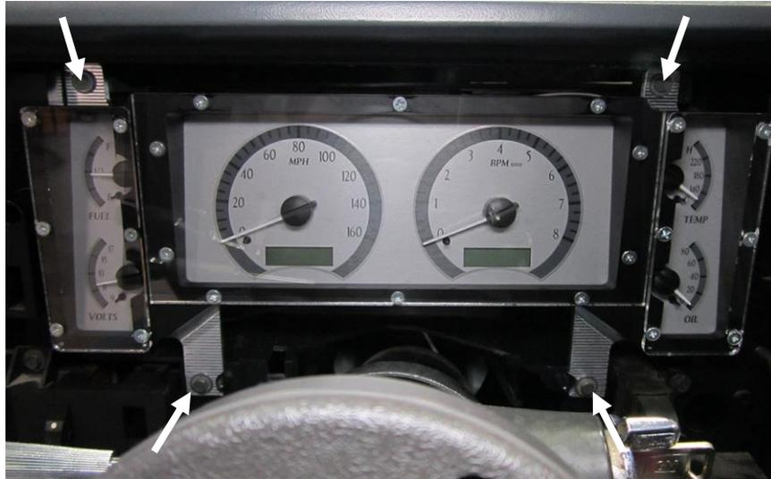
5. Re-install the gauge bezel and refer to the main manual for wiring instructions to complete the VHX installation.
