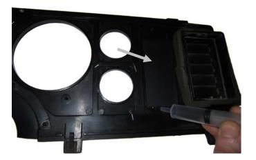
8. Reassemble the stock bezel over the VHX gauges using the three (3) stock screws and once again re-assure fit and alignment. Refer to the main manual for wiring instructions to complete the VHX installation.
