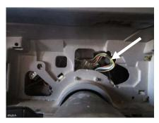
3. Slide the connectors and speedo cable back in the dash structure to clear the VHX gauges.
