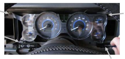
6A. Both the indicator plate and the warning plate will need to be removed from the back of the bezel to allow clearance for the VHX gauges.
