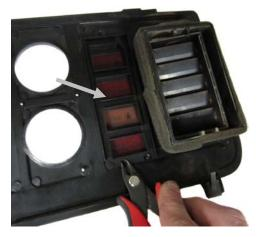
6B. Also the small spacer extrusions on the back side of the bezel will need to be snipped off as shown. Depending on being a GT and/or year of the car the number of extrusions and locations may vary. Any obstruction from the bezel lying flat against the VHX gauges needs to be removed.
