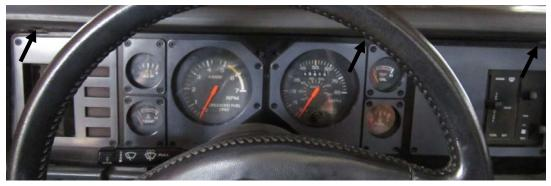
Remove the stock gauge assembly from the dash by removing the four (4) screws and detaching the connector and speedo cable on the back side. Retain hardware for reassembly.
