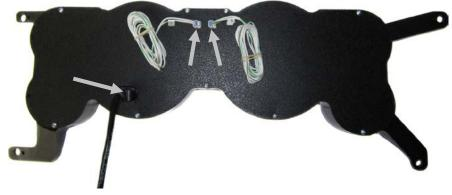
5. Position the VHX gauges over the dash and secure the system by using the four (4) stock mounting screws. There is adjustment in the mounting holes so you can assure alignment by placing the bezel over the gauges before final torqueing.
