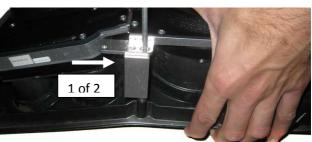
3. Attach the CAT5 cable to the VHX cluster and the two harnesses to use the stock blinker location if so desired. This system comes with two options for the turn signals in your dash. You can either have arrows located in the faceplate of your new VHX display, and/or arrows in your vehicle's stock turn signal locations. To use the new faceplate arrows, follow the wiring instructions for the turn signals found in the main VHX manual.
