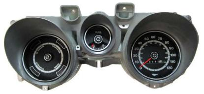
2. Remove the stock gauges and clear lens from the gauge housing. There are nine (9) mounting locations, illustrated by arrows below.
