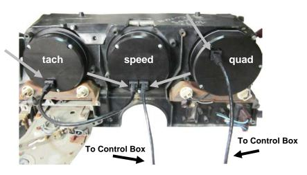
4. Re-install the gauge bezel to the dash housing using the factory hardware and refer to the main manual for wiring instructions to complete the VHX installation.
