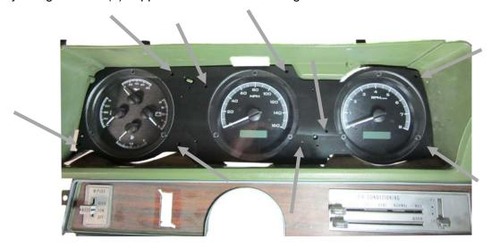
3. Next, you will need to make connections with the provided CAT5 cables. Attach one end of the provided 36" CAT5 cables to both the back of the VHX system speed and the back of the quad gauge with the other ends carefully routed to the control box mounting location. One end of the 12" CAT5 cable goes to the speed and the other end to the tach.
