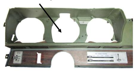
2. With the stock gauges removed, you can now mount the VHX system to the instrument housing by using the nine (9) supplied 3/4" screws in the original screw holes.
