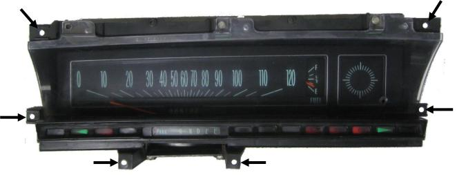
2. Remove the stock gauges, separator plate, and lens from the bezel. The only items to be reused are the original front bezel and two of the six original screws.
