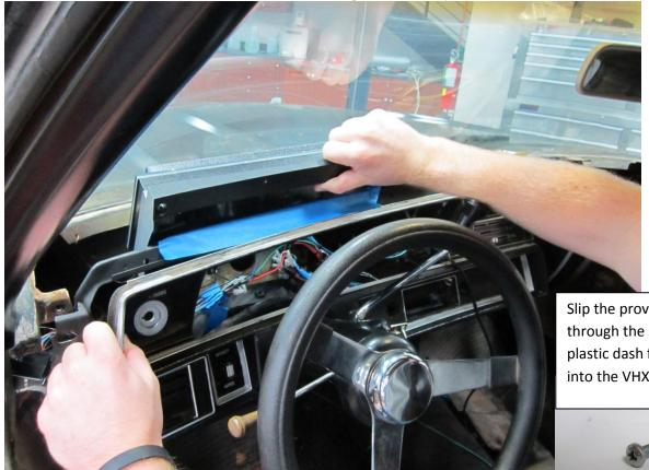
Slip the provided 8-32 screws through the sheet metal dash and plastic dash flange, then thread into the VHX system
