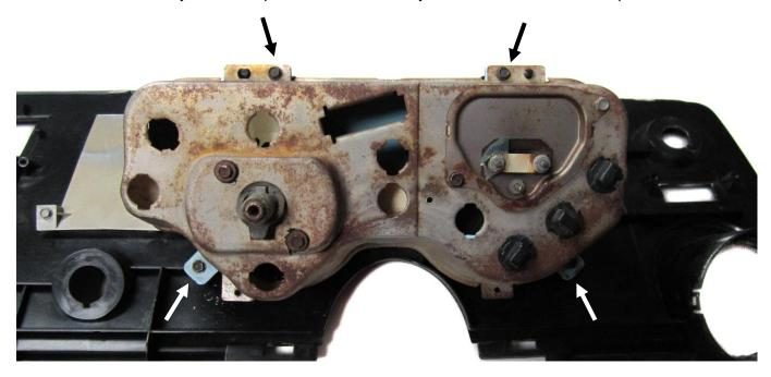
2. Install the Dakota Digital gauge to the factory dash. Using the four screws from step 1, secure the bezel paying special attention to make sure the gauges are properly centered in the bezel opening.
