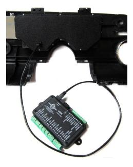
4. Re-install the cluster into the car and refer to the main manual for wiring instructions to complete the VHX installation.
