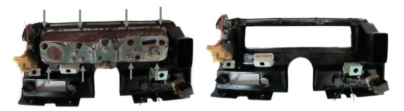
3. With the stock gauges out of the way, place the new VHX gauge assembly in the bezel with the long mounting tabs towards the top. Attach the gauge cluster to the bezel using the stock screws from disassembly.
