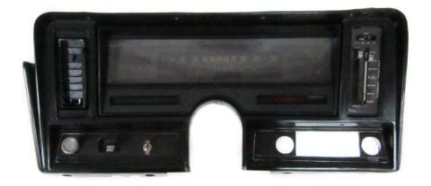
2. Remove the eight (8) screws holding the gauges to the bezel and save the screws for reassembly.
