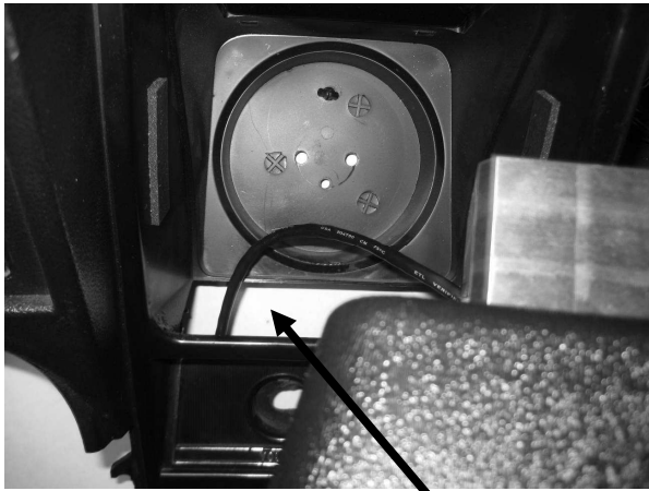
Cable routed through indicator light opening
