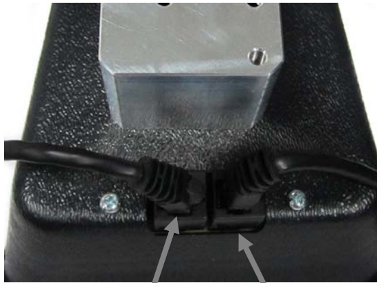
Pre-bend cables to the side before installing so unit will sit flush once inserted into dash
