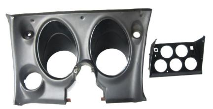
2. Remove the stock gauges, separator plate, and lenses from the bezels. For the main cluster, reattach the lens spacer to the bezel after removing the lens as shown (white arrows). The only items to be reused are the original front bezels and gauge mounting hardware. Now is a good time to clean or refinish the bezels.
