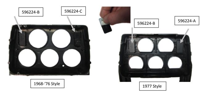
6. With the block-off lens in place, place the VHX center gauges over the back of the center bezel and secure the system by using the four (4) stock mounting screws.
