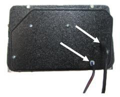
8. The clusters are now ready to re-install into the vehicle using stock hardware. Refer to the main manual for wiring instructions to complete the VHX installation.
