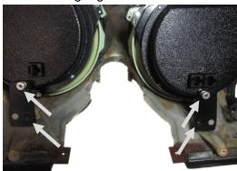
4. Once the VHX gauges are secured to the bezel; connect the 12" CAT5 cable to the Tachometer, and the other end to either port on the Speedometer, connecting the two halves. With the 36" CAT5 cable, connect one end to the open port on the Speedometer, and as the assembled cluster is installed into the dash, carefully route the other end of the cable to the control box mounting location.
