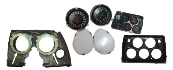
3. The Speedometer and Tachometer are interchangeable side to side. Choose the orientation you prefer, then place the Speed and Tach on the main lens spacers and secure the gauges with the six (6) stock mounting screws. Use two (2) stock mounting screws to attach the ABS plastic brackets to the bezel and thumb screws to secure the brackets to the VHX gauges.
