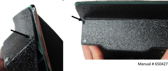
13b. Attach the bezel to the VHX cluster using the original screws from disassembly and the two (2) flat spring nuts provided.
