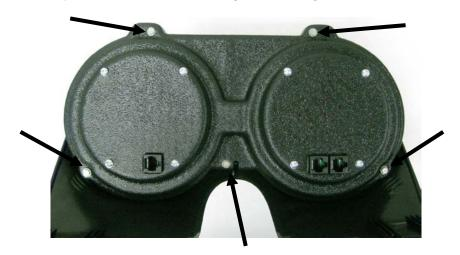
Connect the 12" CAT5 Cable to both halves of the displays and the 36" CAT5 Cable to the extra port as shown. Route the other end of the 36" CAT5 Cable to the Control Box mounting location.
