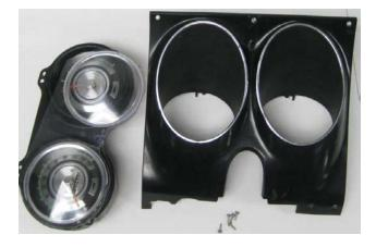
4. For this step, you can re-use the stock foam blocks or use the supplied foam to make replacements for missing or brittle foam pieces. Cut the supplied foam into four small pieces, approx 1.5" long (three inches remaining will be needed for the console gauges). There are four bosses molded in the bezel where the foam should be placed to help prevent any rattles of the lens and bezel.
