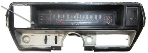
2. Remove the stock gauges from the bezel by removing the four screws shown in grey arrows. These screws are not reused.
