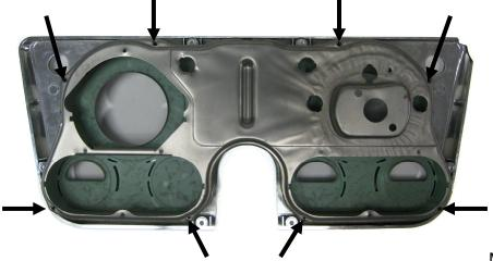
2. Remove the stock gauges, separator plate, and lens from the bezel. The only item to be reused is the original front bezel; the other pieces can be discarded. Now is a good time to clean the bezel and remove any dirt or old lens gasket material.
