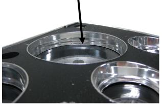
4. Secure the VHX system to the bezel with the eight screws removed from the stock gauges.
