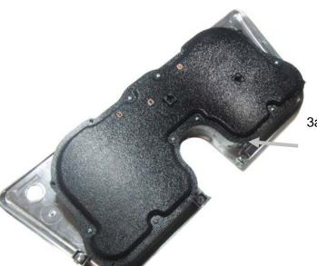
3a. Remove the protective tape from the clear lens and install the VHX system into the bezel. Watch carefully as you insert the system so you don't scratch or damage the lens.
