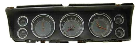
Remove the stock gauges from the bezel and retain the hardware for reassembly. You can also remove the factory clear lens on the front of the bezel or it can be left in place if desired.
