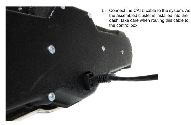
6. Re-install the cluster into the dash and refer to the main manual for wiring instructions to complete the VHX installation.
