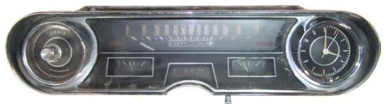
2. Looking at the back of the gauge cluster; remove the clock, speedometer, headlight switch assembly, and mounting brackets so you are left with a bare bezel. Use a 5/64 allen wrench for the set screw at the bottom of the bezel to remove he clock and headlight assembly.
