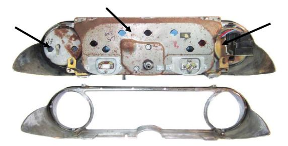
3. Mount the VHX display into the bezel using the four (4) factory screws from disassembly. Connect the 36" CAT5 cable to the back of the VHX display.
