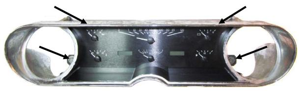
5. Disassemble the clock; the only parts that will be reused are the bezel and the mounting clip. The lens and trim is swaged in place so the tabs will need to be ground down so they can be removed. Pay attention to the mounting clip orientation so it can be reassembled in the same fashion.
