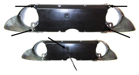
4. Mount the bezel assembly to the dash using the same hardware from disassembly. Take care when routing the CAT5 cable to the control box mounting location.
