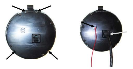
7. Secure the VLC clock assembly and the headlight switch assembly to the stock gauge bezel using a 5/64 allen wrench. Be careful not to overtighten the set screws and take care when routing the CAT5 cable to the control box mounting location.
