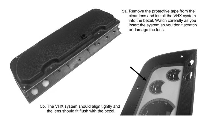
6. Secure the VHX system to the bezel with the seven 6-20 x 1.00" screws and lock washers provided.
