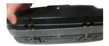
4. Install the VHX system into the bezel. Watch carefully as you insert the system so you don't scratch or damage the lens.
