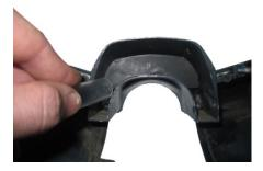
11. Reassemble lower dash bezel when silicone has cured.
