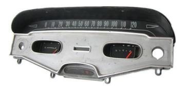
2. Remove the stock gauge housing from the bezel by removing the (8) eight screws on the rear of the metal housing. The only item to be reused is the original front bezel; the other pieces can be discarded. Now is a good time to clean or refinish the bezel.
