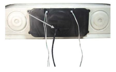
5. The gauge panel is now ready to re-install into the vehicle using stock hardware; take care when routing the CAT5 cable to the control box mounting location. Refer to the main manual to complete the VHX installation.
