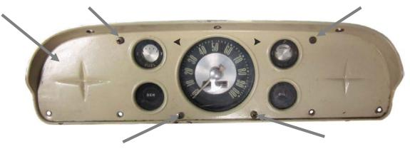
2. Secure the VHX system to the gauge panel using the four screws from disassembly.
