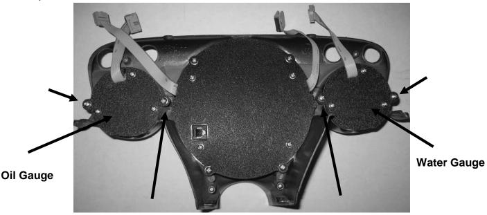
4. Connect the two smaller gauges to the center gauge via the ribbon cable connectors. These connectors are designed to plug in one way to prevent confusion.
