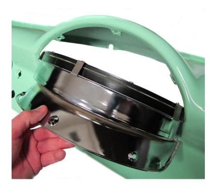
10b. With the bottom of the bezel in place, tip the rest of the system towards the dash hump.
