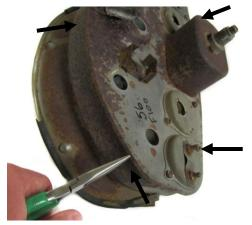
2. Between the shroud and the bezel located on the top hemisphere of the bezel, there are several taps securing the speedometer to the bezel. Using a pliers, bend the tabs straight so the speedometer can be removed.
