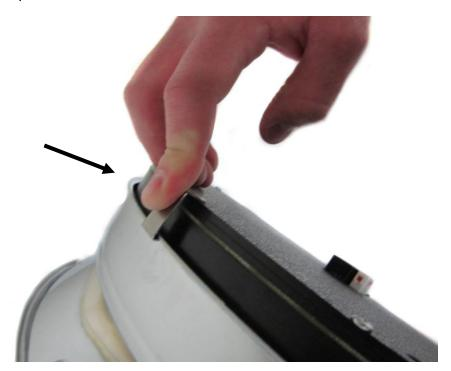
6. Once the holes are aligned, insert the screw/lock washer combination and tighten.
