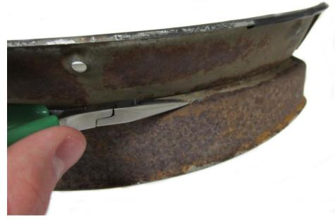
3. Using a pliers once again, bend the metal tab back and forth until it snaps off. NOTE: Some bezels don't have this tab.
