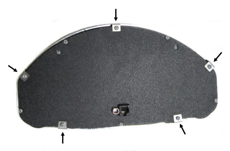
8. As an added form of security, we recommend using RTV Silicone between the perimeter of the Dakota Digital gauge cluster and the factory bezel to prevent vibration and having a better hold.
