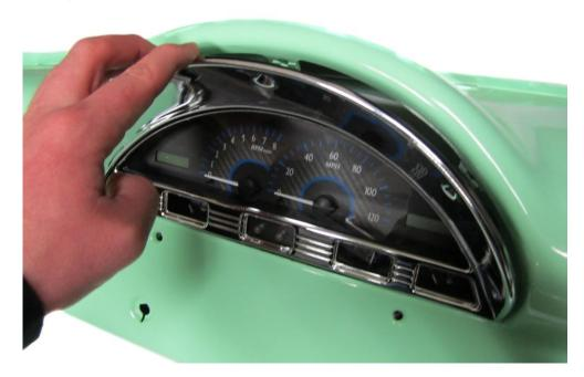
11. Finish securing the assembled VHX instrument system to the dash using the 5 (5) factory oval head screws at the top and bottom of the bezel (black arrows below). Refer to the main manual for wiring instructions to complete the VHX installation.
