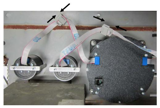
5. Connect the CAT5 cable to the system. As the assembled cluster is installed into the dash, take care when routing this cable to the control box.
