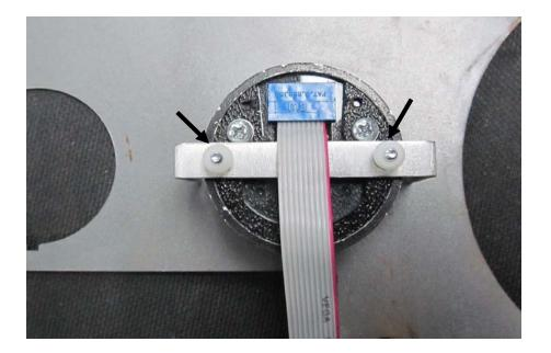
4. Connect the quick disconnect ribbon cables to their respectively labeled counterpart. Note: (OIL-OIL) and (TEMP-TEMP).
