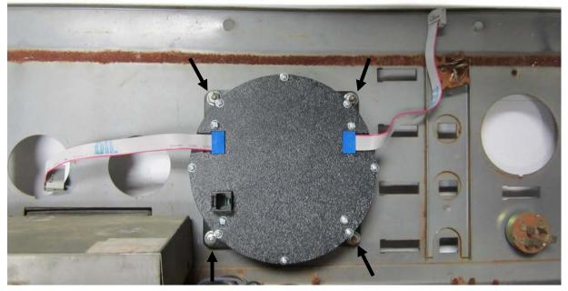
3. Slide the temperature gauge through the opening from the front. Using the provided lock washers, thumb nuts, and bracket, secure the gauge. Pay attention to the orientation of the gauge to keep the gauge at the proper reading level. Repeat this step for the oil pressure gauge.
