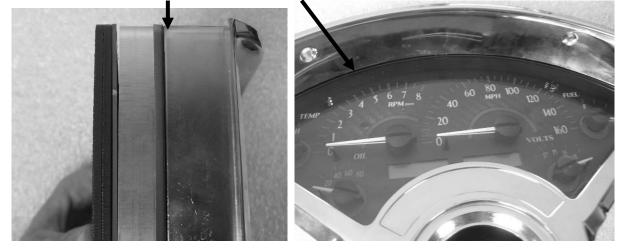
9. Secure the VHX system to the bezel with the six 8-32 x 1.25" screws and lock washers provided.
