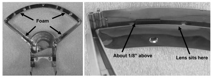
Remove the protective tape from the clear lens and install the VHX system into the bezel. Watch carefully as you insert the system so you don't scratch or damage the lens. The VHX system should align tightly with the bezel and the lens should fit flush with the bezel.
