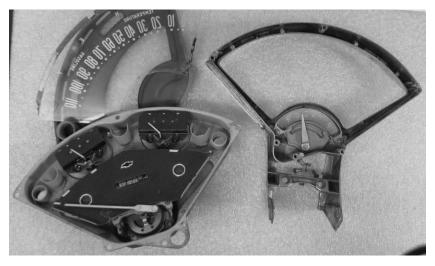
4. For automatic applications, remove the gear position indicator and lens by removing the two screws holding it to the bezel.
