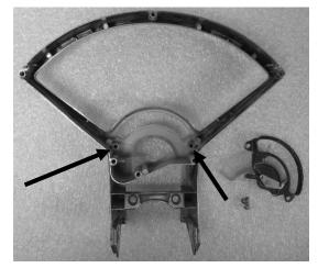
5. For some bezels you will have to grind down the two alignment pegs at the top of the bezel. They must be less than 1/8" tall or the system will not sit flush against the bezel. A grinder or file will work to knock them down a bit.
