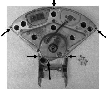
3. Remove the stock gauges, separator plate, and lens from the bezel.
