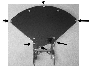
10. Re-install the cluster into the car and refer to the main manual for wiring instructions to complete the VHX installation.
