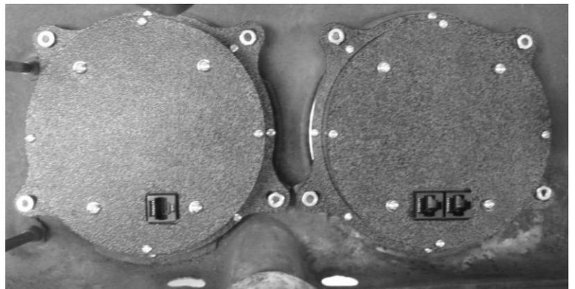
3. Connect the two halves of the new VHX system with the supplied 12" CAT5 cable. Also, route the 3' cable towards the control box location and connect it to the display.
