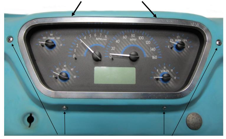
3. Secure the VHX system to the system with the four 10-18x.5" screws provided. The two counter sunk screw are for the upper two locations and the two pan heads are for the lower two locations. Take care when tightening the mounting screws to avoid stripping the threads.
