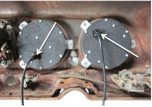
Connect a CAT5 cable to the back of each VHX gauges and take care when routing the other ends to the control box mounting location.
