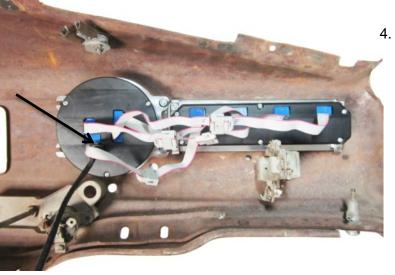
4. Make the proper connections between the four (4) labeled ribbon cables from the Speed/Tach gauge to the lead from each Auxiliary gauge. Example; Fuel cable from the main gauge connects to the Fuel auxiliary gauge cable. Also Connect the CAT5 cable to the back of the VHX Speed/Tach gauge shown with the black arrow. Take care when routing the CAT5 cable to the control box mounting location
