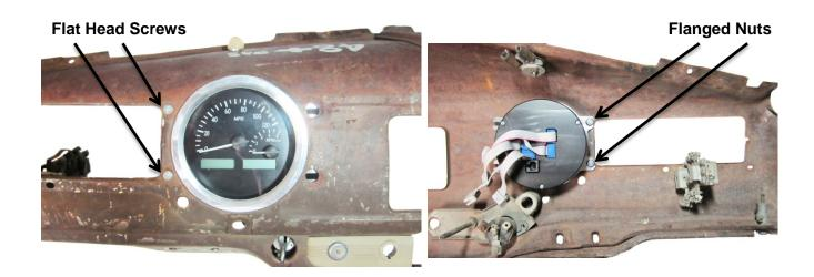
3. Place the VHX Auxiliary gauge into place from the front, use the supplied L-brackets, lock washers, and nuts to secure the gauge to the dash. The direction of the arrow should match the direction of the bracket. Make sure there is no interference from the headlight switch wires and the gauge housing; make placement adjustments if needed.
