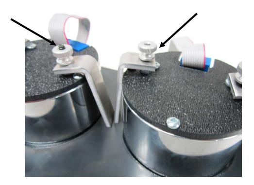
3. Make the proper connections between the four (4) labeled ribbon cables from the main gauge to the lead from each small gauge. Example; Fuel cable from the main gauge connects to the Fuel auxiliary gauge cable.
