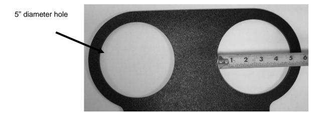
2. Remove the protective tape and insert one of the gauges into a hole and secure using the supplied clamps and thumb nuts. Make sure you align/straighten the system with the dash before you tighten the thumb nuts all the way.
