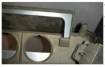
The right side of the dash will be secured by the radio if it exists within the new dash panel. If the radio panel does not exist, holes will need to be transferred from the new aluminum instrument panel, through the factory dash. Screws will then need to be inserted through the backside of the stock dash and threaded into the new dash panel, holding it in place.
