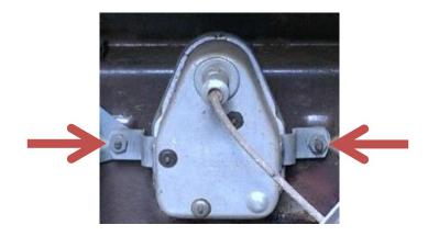
2. Secure the new RLC clock to the dash using the original nuts.
