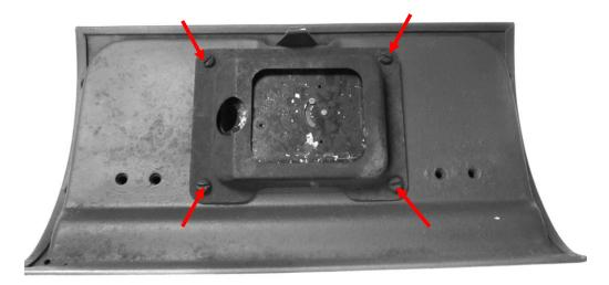
2. Remove the clock assembly and rear housing.
