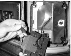
9. Make sure the bulb base is fastened securely in the stock bulb socket. Carefully place the LED assembly onto the housing and press down firmly.
