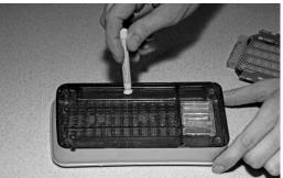
7. Peel the backing off the tape for installation.
