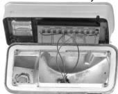
10. Fasten the lens back on with the four original screws.
