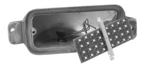
6. Place the new LED assembly into the housing so that the aluminum mounting bracket sits into the groove for the lens gasket.
