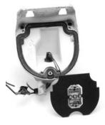
Remove the backing from the tape on the LED assembly and insert assembly into the tail light housing, making sure to keep the assembly centered in housing. Press firmly on the bracket to ensure good tape bonding.
