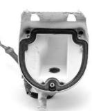
8. Insert the bulb base from the LED assemblies into the bulb sockets. Test the assemblies for tail lights and brake functions to make sure they work as expected before going on.
