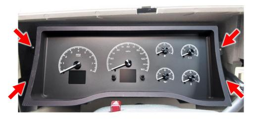
6. Stock style alternators will need an additional wiring connection at the gauge cluster connecter to excite charging. You will need to add resistance from the Pink wire in the A22 location to the Brown wire in the A19 location. The range needed is 500-30 ohms. Three 1/4W 1K resistors in parallel will be in range at 333 ohms. The provided Alternator Load Harness can be used to achieve this.
