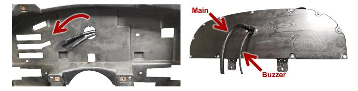
3. Place the HDX system into the dash and secure using hardware from disassembly.
