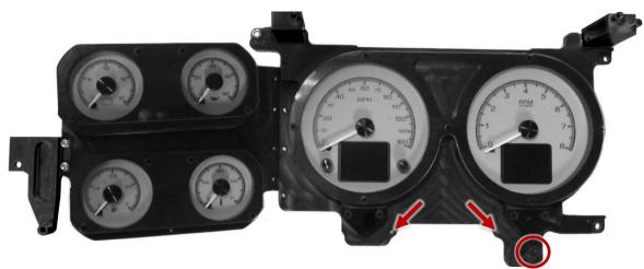
7. Install the stock bezel over the HDX gauge cluster using the stock screws removed in Step One. Tighten the locations shown below first to ensure proper fitment and alignment; if the holes are not aligned correctly, Step Three may need to be repeated.
