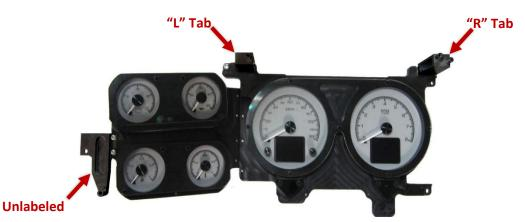
The remaining unlabeled tab goes on the bottom left side of the system, between the satellite gauges. Making sure the countersunk side of the tab is facing away from the rest of the unit, fasten this tab to the HDX system with the two included **6-20 x** <sup>3</sup>/<sub>4</sub>" **flat head screws**. This tab can be tightened until flush.
