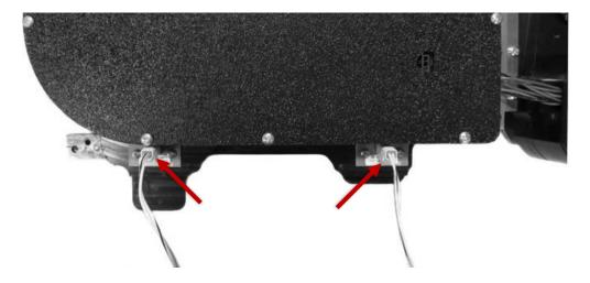
5. Connect the provided main harness and the buzzer (optional for audio feedback) to the back of the HDX system. Carefully route the main harness through the dash to the control box mounting location.
