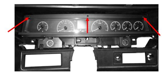
7. Re-install the lower gauge cover using the factory hardware and refer to the main manual for wiring instructions to complete the HDX installation.
