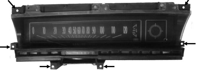
2. Place the system behind the dash from the top side. Be careful to not scratch the system on the dash frame; use tape or a rag to cover sharp areas that could damage the HDX system.
