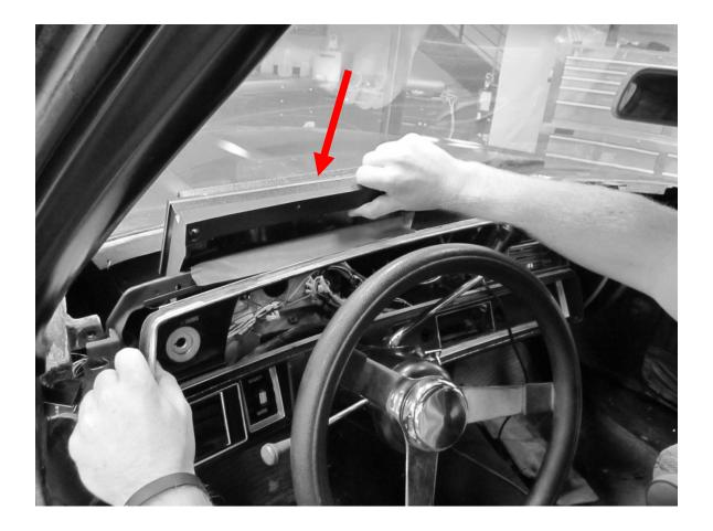
3. Mount the HDX system by sliding the provided screws through the sheet metal dash and plastic dash flange, then thread into the HDX system. Two factory screws will be used to mount the lower portion of the system
