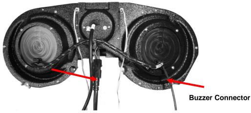
9. Re-install the cluster into the vehicle using the factory hardware and refer to the main manual for wiring instructions and manual 650569 for clock operations to complete the HDX installation.
