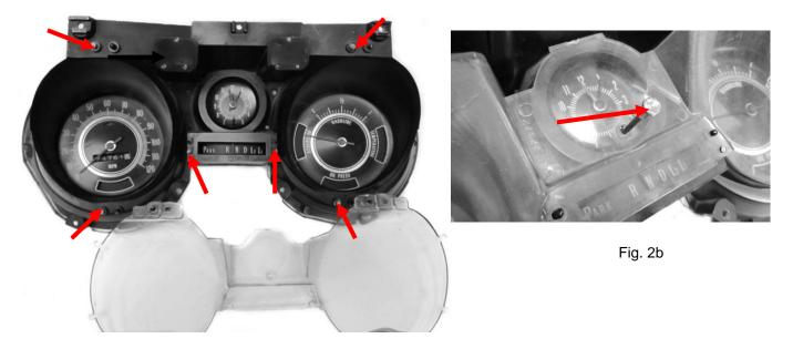
3. Using the provided screws; attach the Speed and Tach instrument panels to the stock instrument housing.
