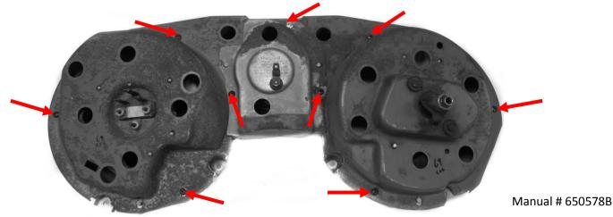
2. Remove the stock lens using a pair of side cutters or a utility knife; the original lenses will not be reused. Using a small flathead screwdriver, remove the clock adjustment screw to allow lens to be lifted off of the housing (Fig. 2b.)
